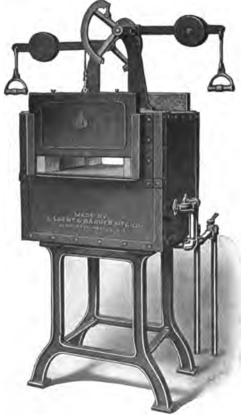
Fig. 193. Double Door Furnace for Heating and Annealing Work Courtesy of Gilbert and Barker Manufacturing Company, Springfield, Massachusetts
